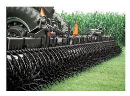
**TINE WEEDER** – The 45° tines are more effective at uprooting weeds than they are for covering them. The longer tines are better able to follow the surface of the soil so that they loosen the soil evenly. The tines assist with removing shallow germinated weeds that are in the crop row without disturbing the planted crop.
